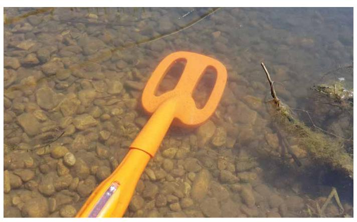
at depth, it will work instantly. In water 10–30m deep it needs to be activated. You simply tilt the Scuba Tector on its end and back three times. You'll get a confirmation signal and it's ready to go. Most pleasure diving is done in the first 30m but it's good to know that it's over engineered for the task in hand.
